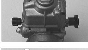
Remove the main jet 2, the main jet holder 3 and the baffle 4.
