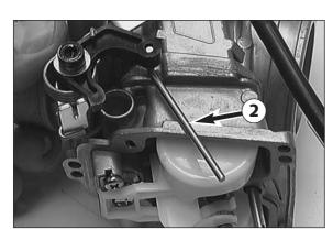
Engage the push rod ② of the accelerator pump at the lever.
