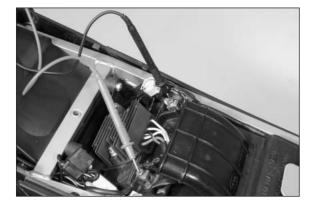
**Regulator rectifier output** – measure the voltage with the measuring leads of the peak voltage adapter directly on the poles of the vehicle battery:
