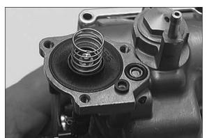
Turn the carburetor around, remove the 3 screws and remove the cover of the accelerator pump.
