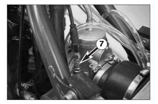
To adjust, remove the seat and the gastank, push the protective cover upwards, loosen the counter nut and turn the adjustment screw O accordingly. Turn the adjustment screw clockwise for more play or anticlockwise for less play.
